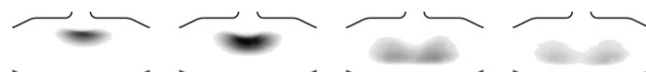
Fig. 6. The influence of the sample gas flow on flames in a type S2 system at 11.3 ml/min oxygen flow. The flames correspond to the sample gas flows from Fig. 5 starting at 2.0 ml/min. Hydrogen (+ sample) is supplied from the top and oxygen from the bottom.
