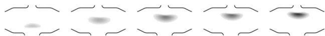
Fig. 4. The influence of the oxygen flow on the brightness of flames in a type S2 system. The flames correspond to the oxygen flows from Fig. 3. Hydrogen (+ sample) is supplied from the top and oxygen from the bottom.
